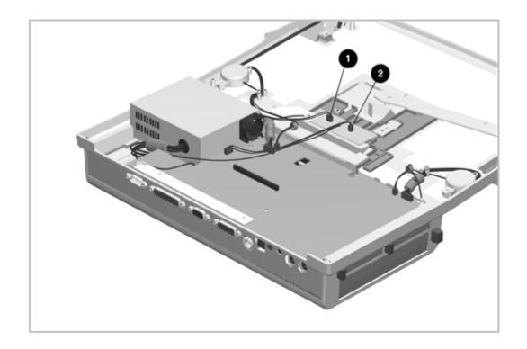
Figure 6-16. Disconnecting the Fan Control Board
